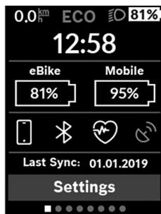
As well as the status bar, the status page also shows you the current time and the state of charge of all your eBike's batteries, as well as the state of charge of your smartphone battery if the smartphone is connected via Bluetooth®. It may also display symbols to indicate an activated Bluetooth® function or a device connected via Bluetooth® (e.g. a heart-rate monitor). You will also be
